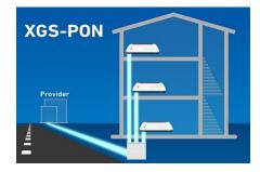
XGS-PON (10 Gigabit Symmetric Passive Optical Network) XGS-PON accelerates data transmission in GPON infrastructures to speeds of up to 10 Gbit/s, optionally in both transmit and receive directions.
